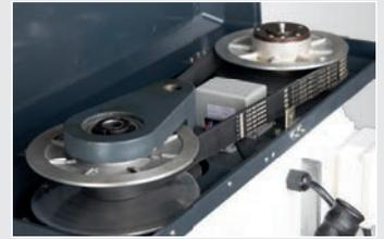
**STUFENLOSES MECHANISCHES GETRIEBE**
