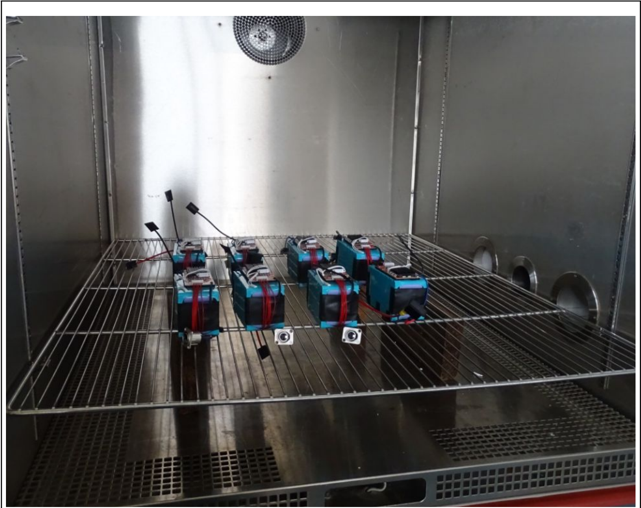
Fig. 2.2 Batteries in T.2 Ref.1 and Ref.2b, §7.2.2 Ref. 2a Test setup (Thermal test, case stress)
