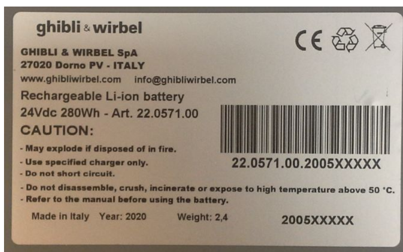
Fig. 1.2 SDI INR 18650-29E 7S4P In the case
